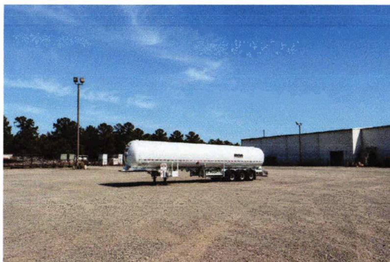
► 30,000-gallon storage tank
